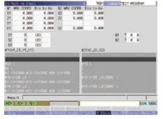
**On-machine program check function** Using manual handle feed, operations can be run in the forward or reverse directions, and you can temporarily stop program operation, edit the program, and then restart operation.
