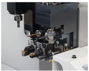
The back tool post on Type X and XII machines can accommodate a total of 8 tools: 4 rotary tools in the upper row and 4 fixed tools in the lower row.
