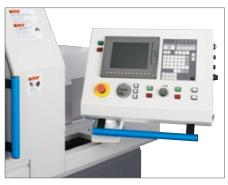
**Position adjustable operation panel** By swiveling the position adjustable operation panel, you can perform operations while viewing the machining area.
