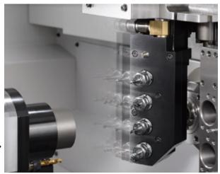
Features a B axis for rotary tools on the gang tool posts of Type IX and XII machines as standard; it can be set over a  $135^{\circ}$  range from  $90^{\circ}$  to  $-45^{\circ}$ .
