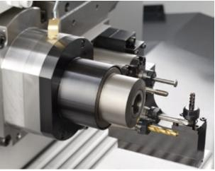
For the opposite tool post, a tool post that is capable of pinch milling or one that can handle deep hole machining can also be selected as options.
