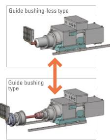
Ability to use as a guide bushing type or guide bushing-less type by switching between them
