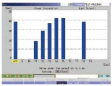
**Eco screen (example graph display)** The machine's power consumption can also be shown in the form of an easy-to-understand graph.
